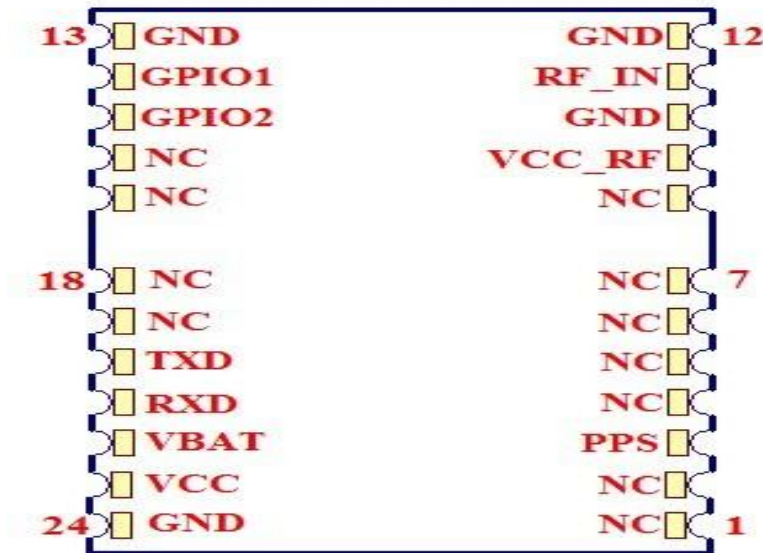
Figure 2: GT-1612-MTR Pin Package
